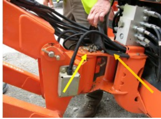
Cover plate and sheared bolts
